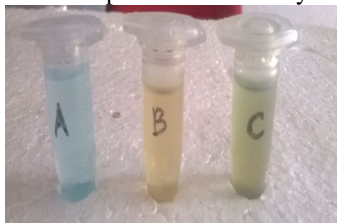
Figure 1. Synthesis of copper nanoparticle A -Cu solution, B -leaf extract, C -Cu solution + leaf extract
