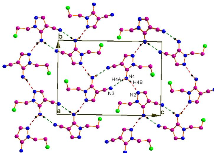
**Figure 2.** Packing of the molecules in crystal of the compound ( $C_6H_7ClN_4$ ). Dotted lines indicate, N-H...N intermolecular interaction; the hydrogen's are omitted for clarity
